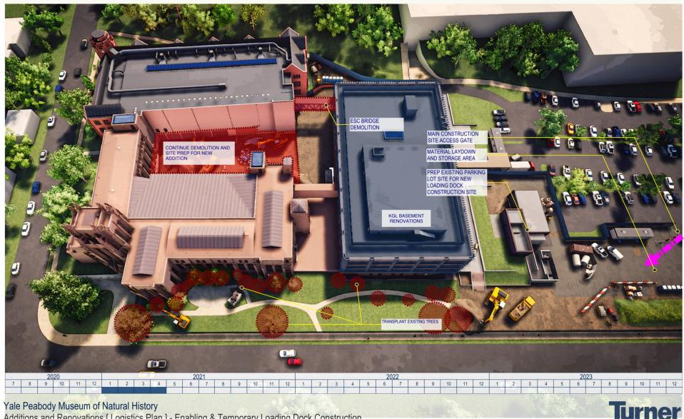
Additions and Renovations [ Logistics Plan ] - Enabling & Temporary Loading Dock Construction
