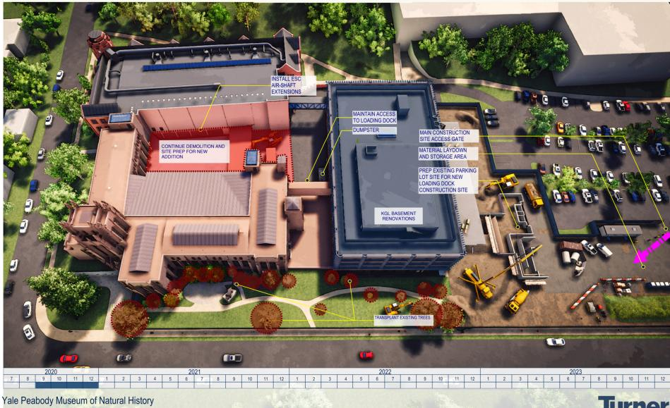
Additions and Renovations [Logistics Plan] - Enabling & Loading Dock Construction
